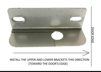
The bracket set contains a Top and Bottom bracket. The Top bracket is stamped with the letter "T". The Bracket set is also directional and must be installed in the correct direction shown in the above photos. If the bracket set is installed the wrong direction the linkage rods will bind.
