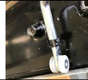
4D - With the bracket loose press the Plastic Bushing in the Bracket.
