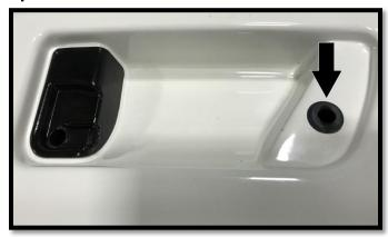
Step 3 – Install Door Handle (TB-37-93-949), The Plastic Washer (TB-1622-WASH) and Linkage Assembly (TB-1622-LINKAGE).
