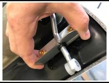
Step 5 – Install the 2 Door Hinges (TB-37-93-295) with the 4 M6 Screws (TB-37-51-2759).
