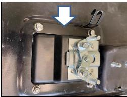
() Tighten all 4 button head scews. Please note, a Allen head wrench will be needed to hold button head screws as you tighten nylon lock nuts.
