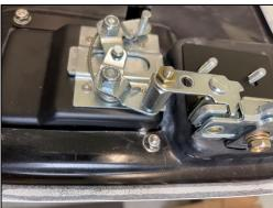
6 – Install 2 Nylon lock nuts (TB-37-55-7007) to lower latch bracket (as shown below) and tighten.
