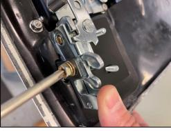
5 – Install the Adapter Nut (TB-37-93-5008N) Using a  $\frac{1}{2}$ " Wrench and Nut Driver tighten the Adapter Nut (as shown below).
