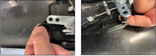
B) Insert the "L" shaped end of Cable into the Clip Retainer (as shown below) and rotate Clip Retainer until in snaps onto the Cable's "L" shaped end (this will be a tight fit so using pair of needle nose pliers will help the clip snap onto the cable).
