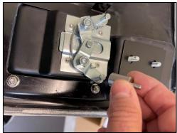
3 – Set Lower Latch (TB-37-93-5007A) onto Adapter Standoff (as shown in photo below). Align Lower Latch with Door Bracket as shown\_\_\_\_\_
