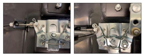
F) Secure the Cable Assembly with the 2 Zip Ties located on the door (see photos below).
