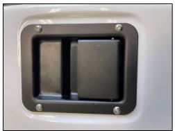
A) Install the 2 bottomhead screws first (leave screws loose). The upper 2 button head screws will be installed with the cable bracket (TB-37-93-5013).
