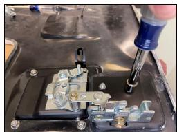
7 - Install 2 machine screws (TB-37-51-2759) into the Upper Latch Bracket (TB-37-93-5007B) as shown below and tighten screws with a Phillips head screw driver.
