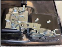
4 - Install 2 machine screws (TB-37-51-2759) into the Lower Latch (as shown in photos below) and tighten the screws with a Philips head screw driver.
