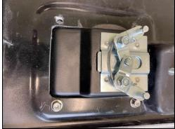
B) Install the cable bracket (TB-37-93-5013) along the upper 2 button head screws for door handle.
