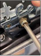
8 – Install 2 Nylon lock nuts (TB-37-55-7007) to Upper latch bracket (as shown below) and tighten.
