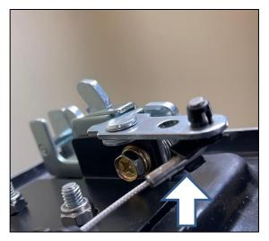
C) Press the plastic Cable end into the Upper Latch Bracket until it snaps into bracket (see photos below)
