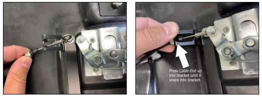
E) Insert the Cotter Pin (TB-37-93-5349) into the Latch Assembly (as shown in photo below). Using a pair of pliers bend the cotter pin to hold Cable on the latch (see photo below).
