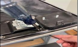
2 - Place Adapter Standoff (TB-37-93-5008S) onto lower latch peg.
